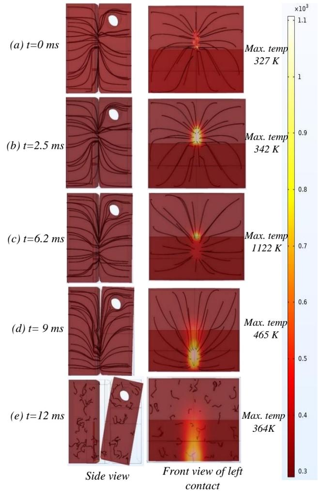
Fig. 7. Temperature and current stream on the contact surfaces.
