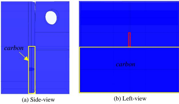
Fig. 5. Contact area Cu-C contacts in closing position.
