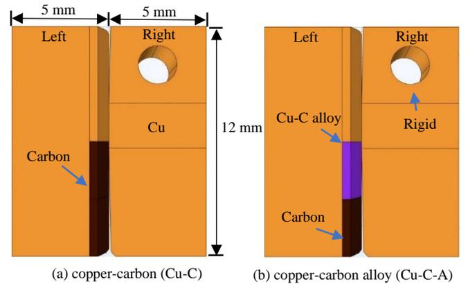
Fig. 1. Two contacts with different materials used in simulation.
