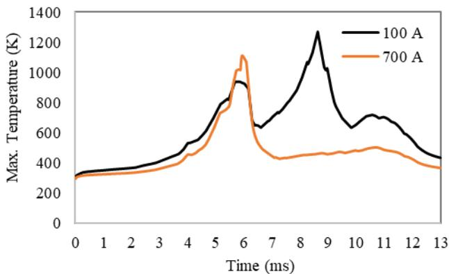
Fig. 8. Maximum temperature of Cu-C contact for 700 A, and Cu-C-A contact for 1000 A.
