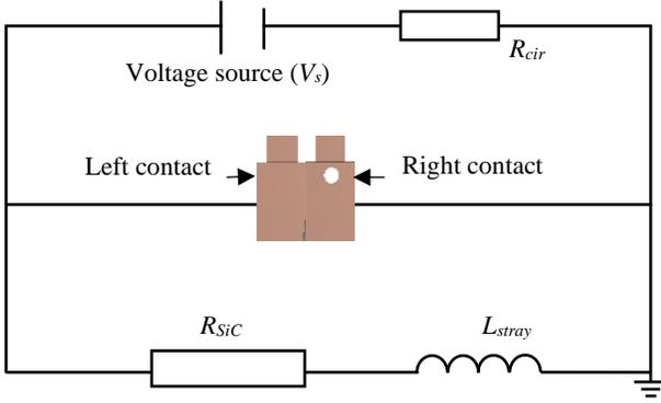
Fig. 2. Electrical circuit diagram of contact model connection.
