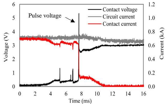
Fig. 10. Experimental waveforms of voltage and current of Cu-C contact for 700 A [6].
