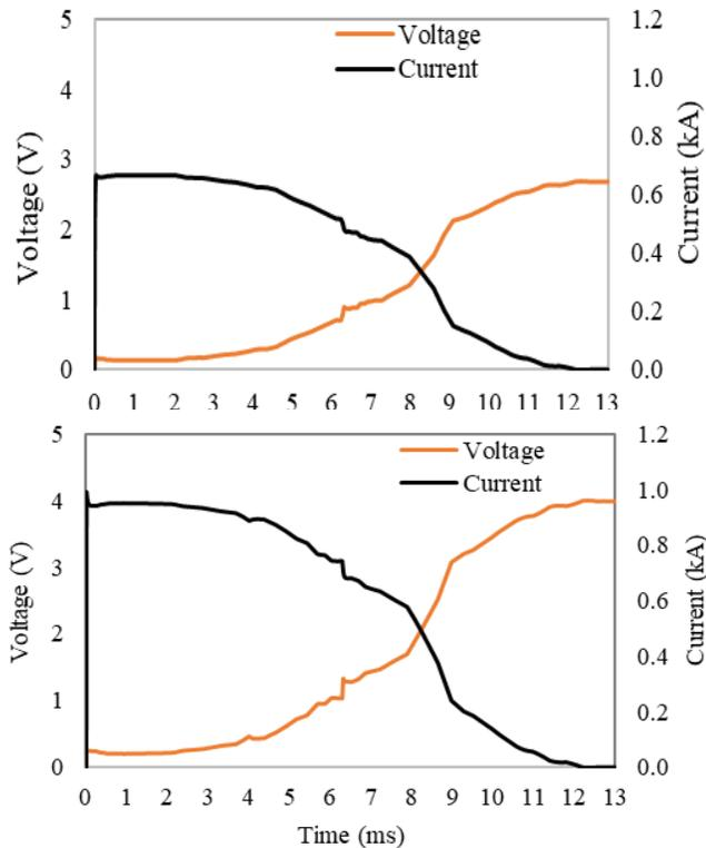
Fig. 12. Contact voltage and current of Cu-C-A contact for 1000 A.
