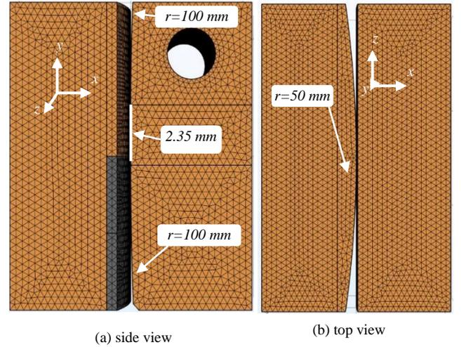
Fig. 4. Mesh and curvature along the contact surface in front view.
