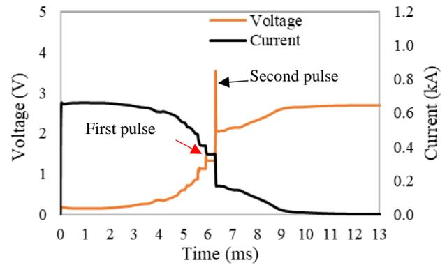
Fig. 9. Contact voltage and current waveforms of Cu-C contact for 700 A.
